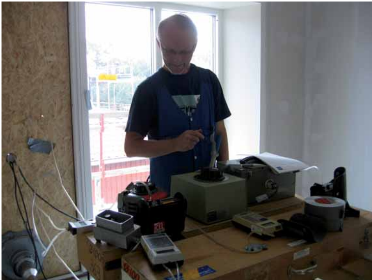
Figure 4.19 Ingmar Nilsson of SP measuring the air leakage.
